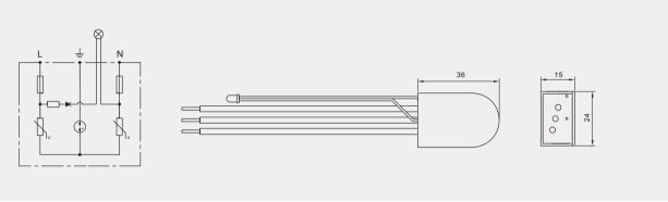
■ Type 3 surge arrester is installed between LPZ2 and LPZ3, it can provide protection for equipments.
